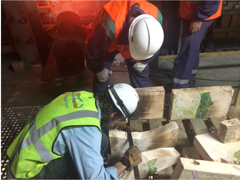
Figure 7 Vidrala and PaneraTech team measuring actual wall thickness after the recovery of the blocks. .....
