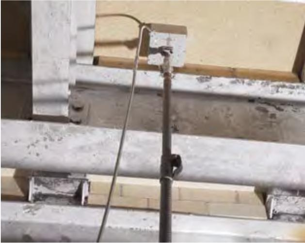
SmartMelter portable sensor collecting data on a furnace bottom.
