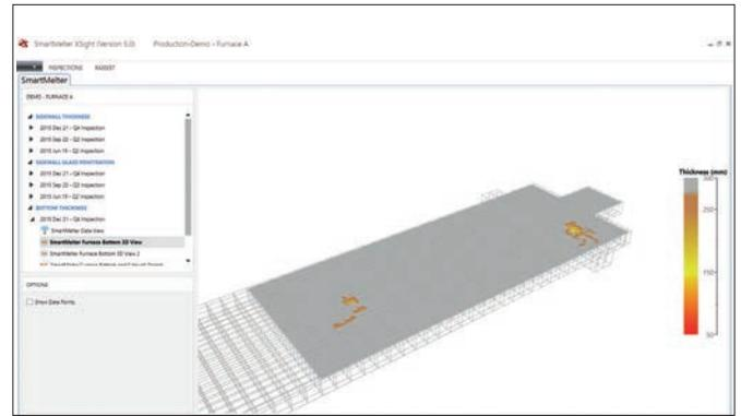
drain and measurements were compared. The actual block was found to be within 4mm of SmartMelter's measurements.
