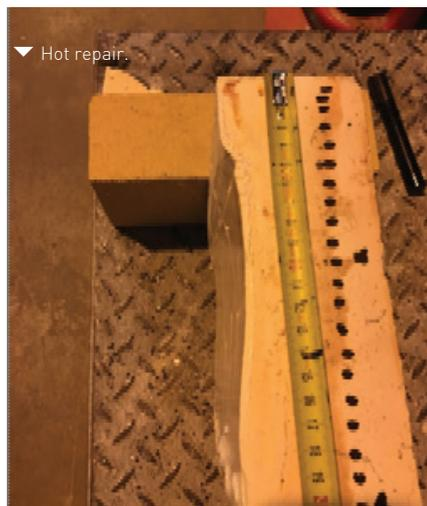
fused-cased AZS, high zirconia or Chrome refractories. The interface between the glass and the wall is recorded to produce a measurement of the residual refractory thickness. The Furnace Tomography Sensor (FTS), used on furnace bottom and sidewalls, operates from the outer layer of insulation. The FTS maps early-stage glass penetration and measures the residual thickness of the insulation and refractory layers.
