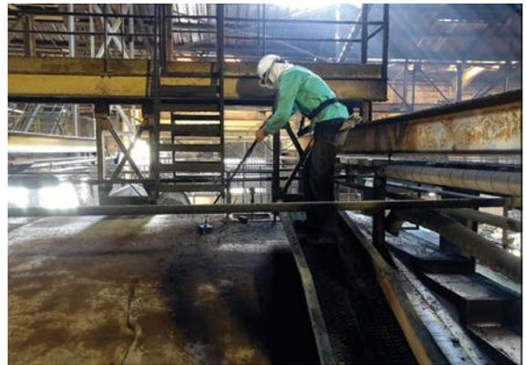
SmartMelter inspection of a furnace crown.
